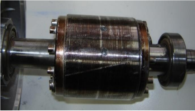
Fig. 6. Rotor with two broken bars.
