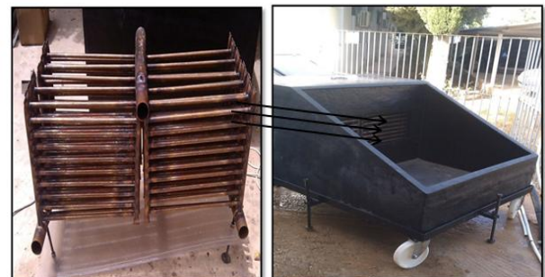
Figure.4. Photograph the condensing chamber and photograph of the experimental setup.
