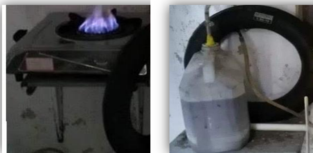
Fig. 13: Use of biogas as natural gas for cooking and lighting.
