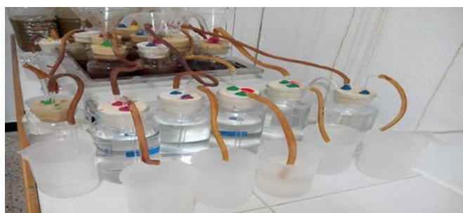
Fig. 1: Experimental set-up of the six digesters linked to the gasometers.
