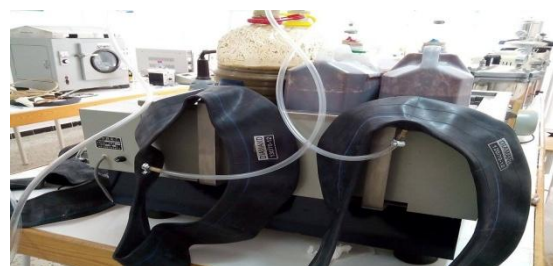
Fig. 2: Experimental set-up of the three digesters linked to the air tubes.
