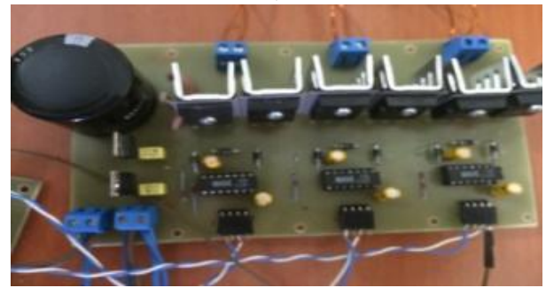
Fig. 19: Photograph of the MOSFET driver
