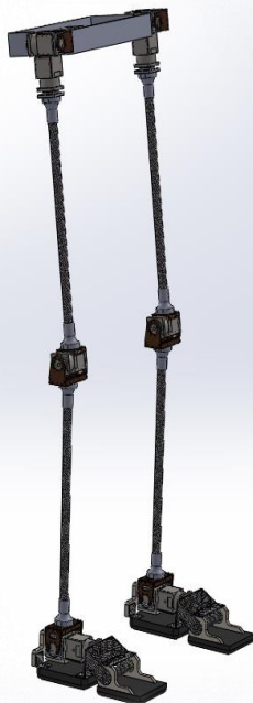
Fig. 1. An Isometric View for the Two Biomechanical Legs Designed with Solidworks.
