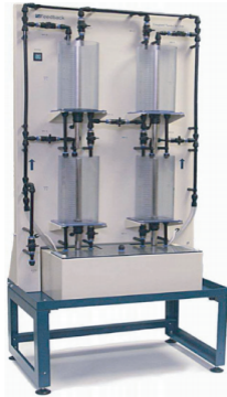
Fig. 6. Plant of four coupled tanks [26]
