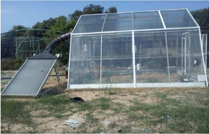
Fig.1: Pictorial view of the solar greenhouse dryer
