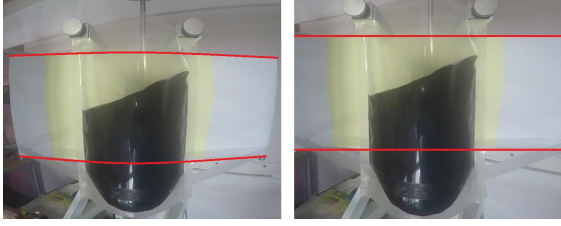
Fig. 5. Original image (left) and undistorted image (right). Note the shape red lines corresponding to top and bottom edges of the back white screen, before and after the undistortion
