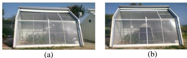
Fig.1 Photo of the experimental greenhouses: (a): Insulated greenhouse (IG), (b): Insulated greenhouse with latent heat system (IGHLS).
