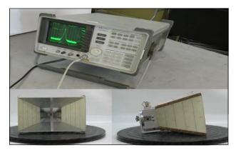
Figure 1. Double- ridged waveguide horn antenna with spectrum analyzer
