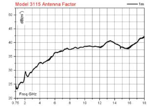
Figure 2. Model 3115 Typical Antenna Factor
