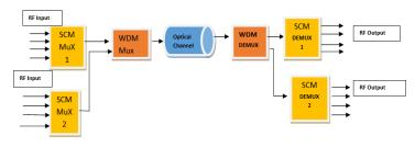
Figure.5. the architecture of SCM/WDM
