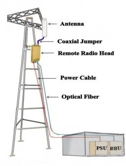
Figure.4. the architecture of FTTA.
