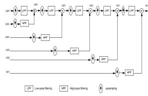
Fig. 4 The Inverse DWT filtering process
