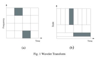
Wavelet transform can give more reliable and detailed time-scale representation for it more than the short time Fourier transform.
