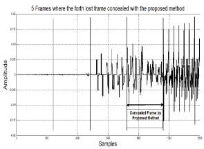
Fig.4 Concealed frame excitation by the proposed PLC method.
