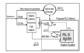
Fig.1. Scheme of the proposed PLC method of the modified ACELP decoder.
