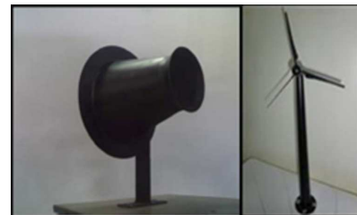
Fig. 1 Design of the tested diffuser and the small-scale horizontal axis wind turbine.
